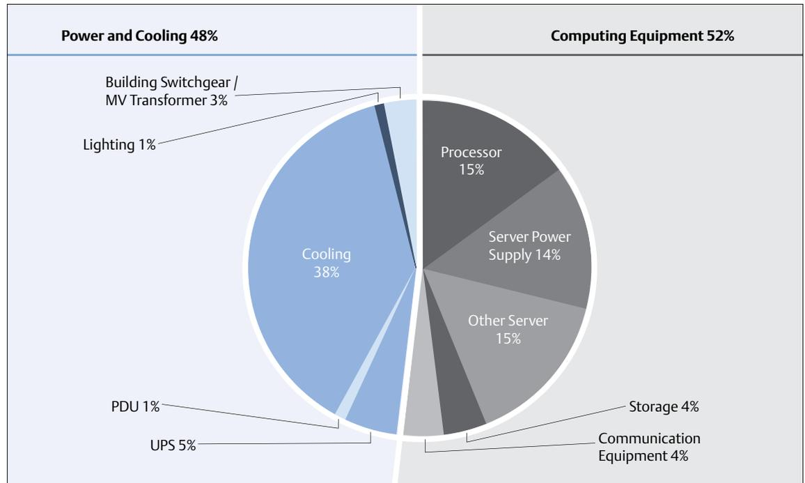
**Figure 1. Typical power draw in a data center.**
